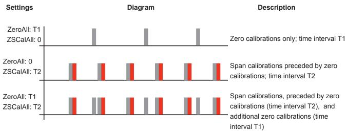
Fig. 7-8: Graphical Explanation of Interval Time Settings
